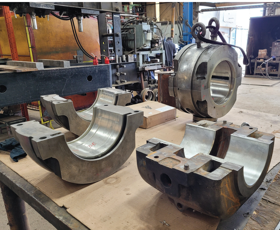
Davis Machine produces babbitt bearings in diameters from 2 in. to 10 ft. for pumps at pipelines, coal plants, hydro dams, or natural gas turbines.
