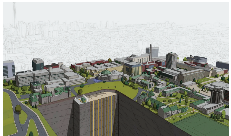
A rendering of the new geoexchange the University of Toronto is constructing 250 metres below King's College Circle at its St. George campus in downtown Toronto.
